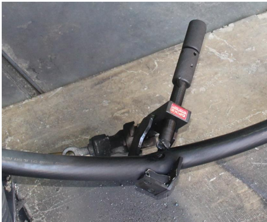
Figure 8-9: Test 3237: Grounded SPIKE tool with ball-stud at 27 kA fault, 15 cycles.
