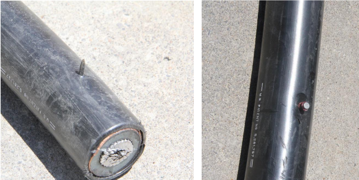
Figure 8-4: Nail punctured through on 28 kV, 1000 kcmil aluminum conductor
