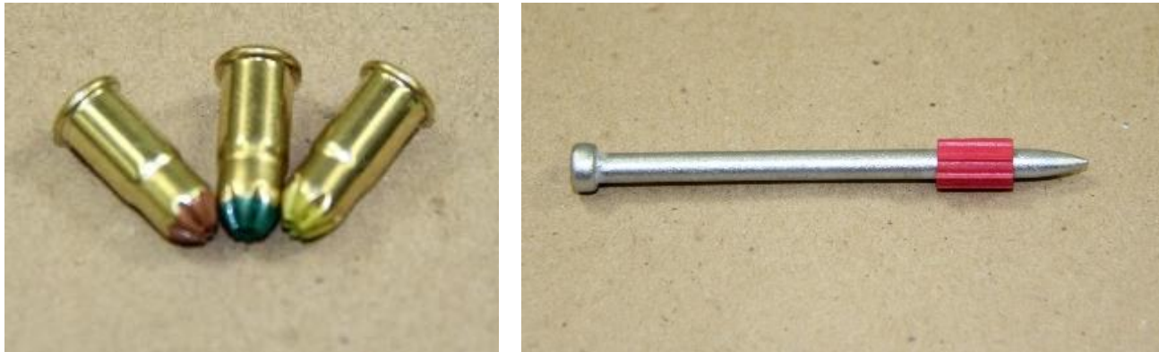
Figure 5-2: Cartridge and hardened nail supplied with SPIKE.
