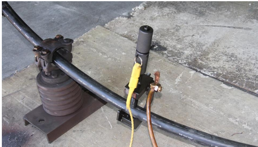
Figure 6-2: Setup of grounded SPIKE tool using split-bolt.
