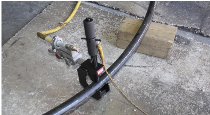
Figure 6-3: Setup of grounded SPIKE tool using 25 mm ball-stud.
