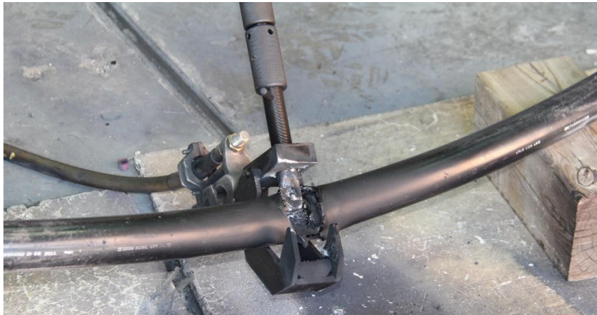
Figure 8-10: Test 3238: Grounded SPIKE tool with ball-stud at 19 kA fault, 15 cycles.
