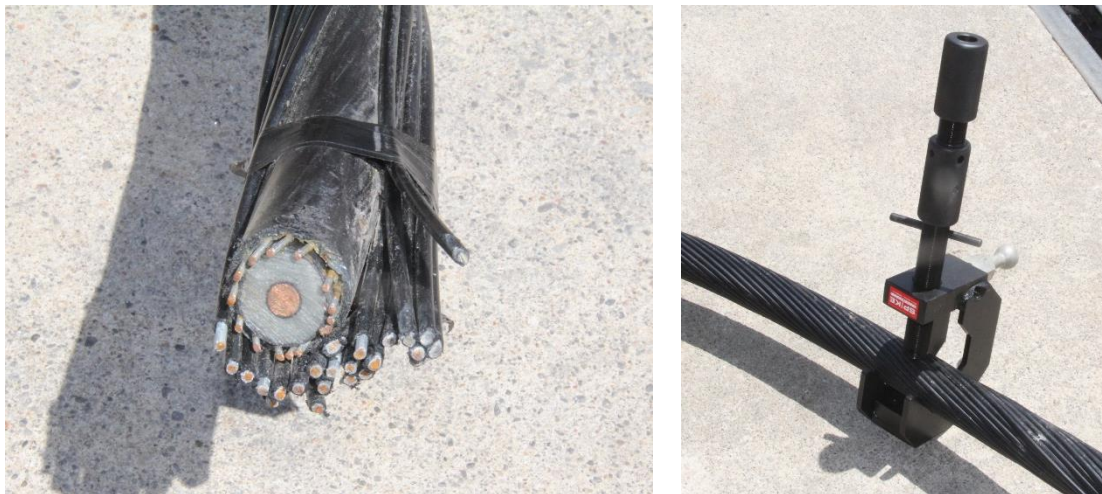
Figure 8-1: SPIKE installed on steel armoured cable.
