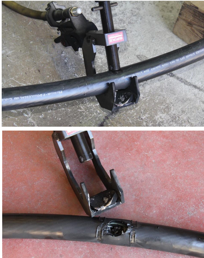
Figure 8-8: Test 3236: Grounded SPIKE tool with ball-stud at 13.8 kA fault, 15 cycles.
