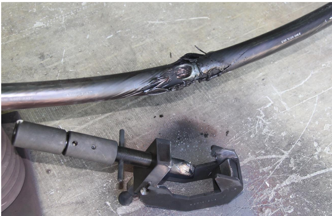
Figure 8-6: Ungrounded SPIKE tool with 13.8 kA fault, 15 cycles.
